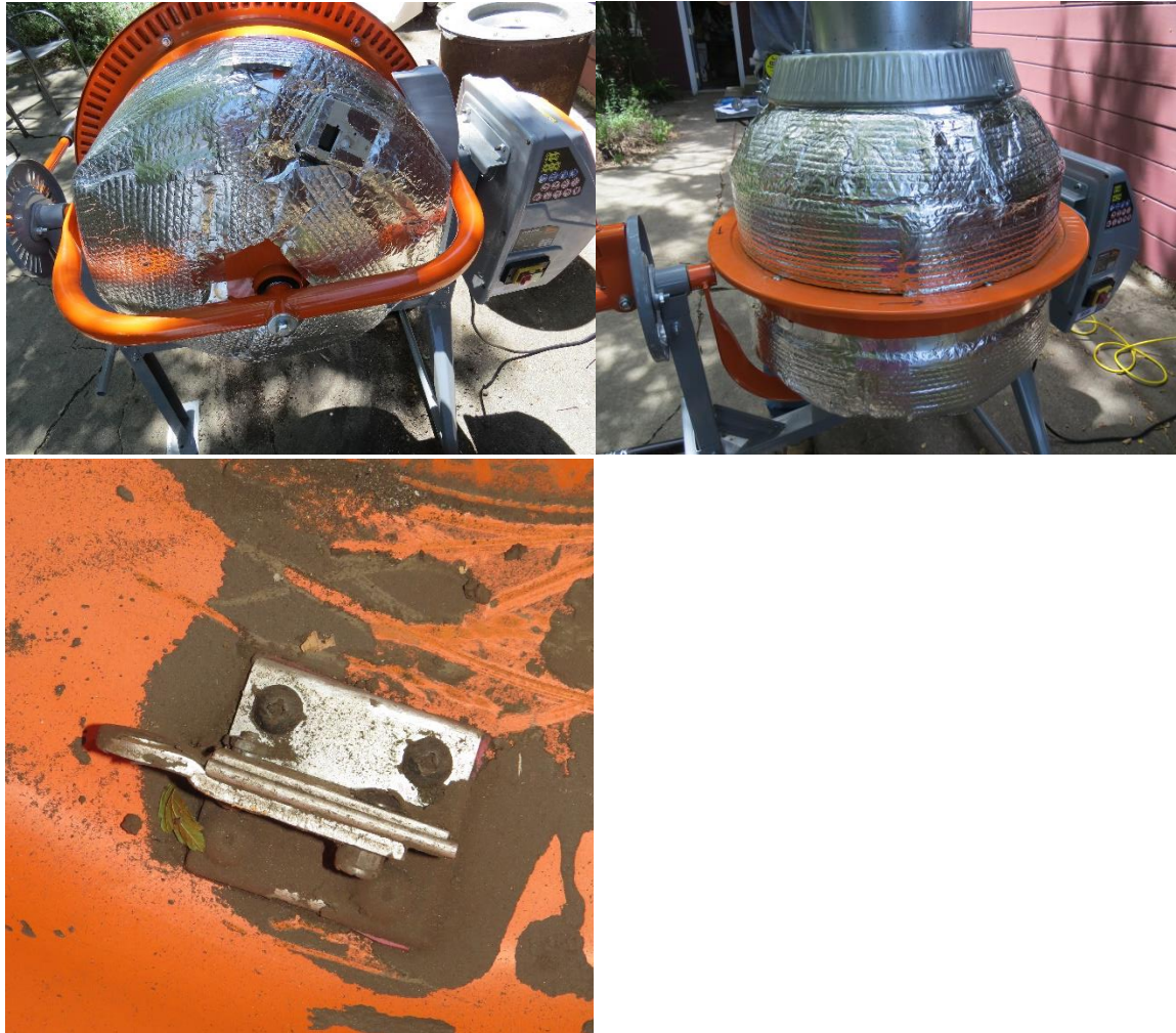
Figure 2. Top – Cement mixer with insulation (top) and Elitech® RC-4 temperature logger attached to the bottom of the drum (top right). Insulation on the bottom of the mixer is shown at top left, with attached data logger visible. Top right shows the fully-insulated mixer drum. The external probe of the temperature logger was inserted into a hole drilled into an aluminum angle assembly (bottom) that was bolted to the inside of the drum about 6 mm from the bottom welded seam. The temperature logger was downloaded after each set of tests on a given day was completed.
