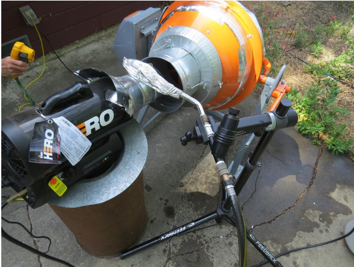
Figure 4. Full equipment setup including mist nozzle suspended by a bike stand. A drip irrigation filter was plumbed into the water supply to help screen out debris that might clog the nozzle. The mist nozzle is covered with an aluminum heat shield. Metal pipe and fittings were needed in the area exposed to the hot air exiting from the mixer. In this image, the mixer drum is only partially covered with insulation. During operation, a handheld IR thermometer (upper left in image) was used to monitor temperature.
