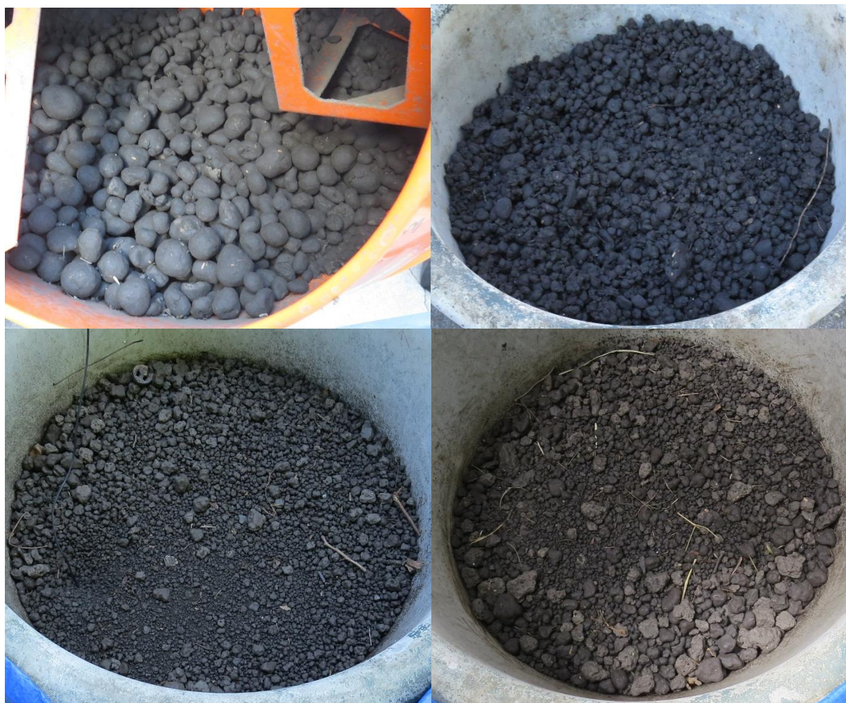
Figure 9. Capay silty clay loam soil after heating and mixing in the cement mixer. Top – In trial 1, the soil was initially quite dry (6% volumetric water content) and water was added during the heating/mixing process using the mist setting of a hose end sprayer. Too much water was added in this first trial and the overly wet soil balled up into large, rounded aggregates as seen in the mixer (left; largest aggregates have accumulated at the surface) and after transfer to the holding vessel (right). Bottom – minimal balling of soil but rounding of small aggregates is seen in heat treated soil from trials 15 (left) and 11 (right).
