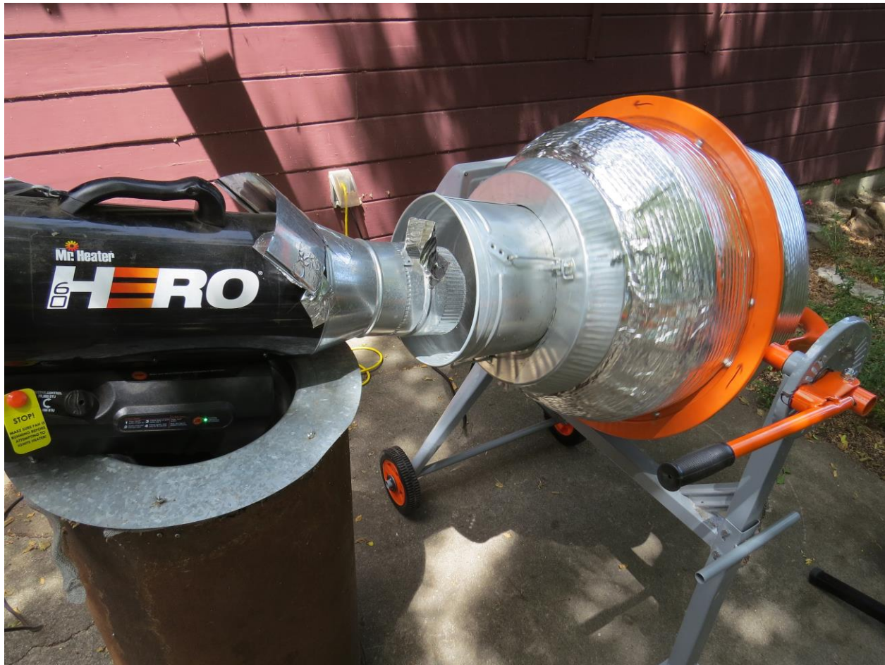
Figure 1. Equipment set up used for heat treatment trials. The Mr. Heater 60 Hero® propane heater (left) has been modified by attaching a reducer and short length of ducting to direct hot air into the mixer while allowing the unit to remain further from the exiting hot air stream. The opening in the top of the ducting is for mist injection (Section 2.1.3). A heat shield has also been added to deflect hot air away from the plastic handle. The heater rests on a drum with a depression in the lid that allows the heater to be tilted. A detachable collar at the opening of the cement mixer (Yardmax® 4 cu. ft. electric cement mixer) allows the mixer to be close to a horizontal position to improve agitation of the soil mass without losing soil out the opening.
