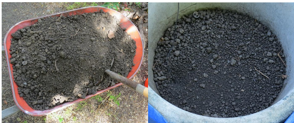
Figure 17. Left, soil was collected into a wheelbarrow and mixed to degree possible. Large clods were broken up, root fragments were left in place. Right, soil appearance after heating.
