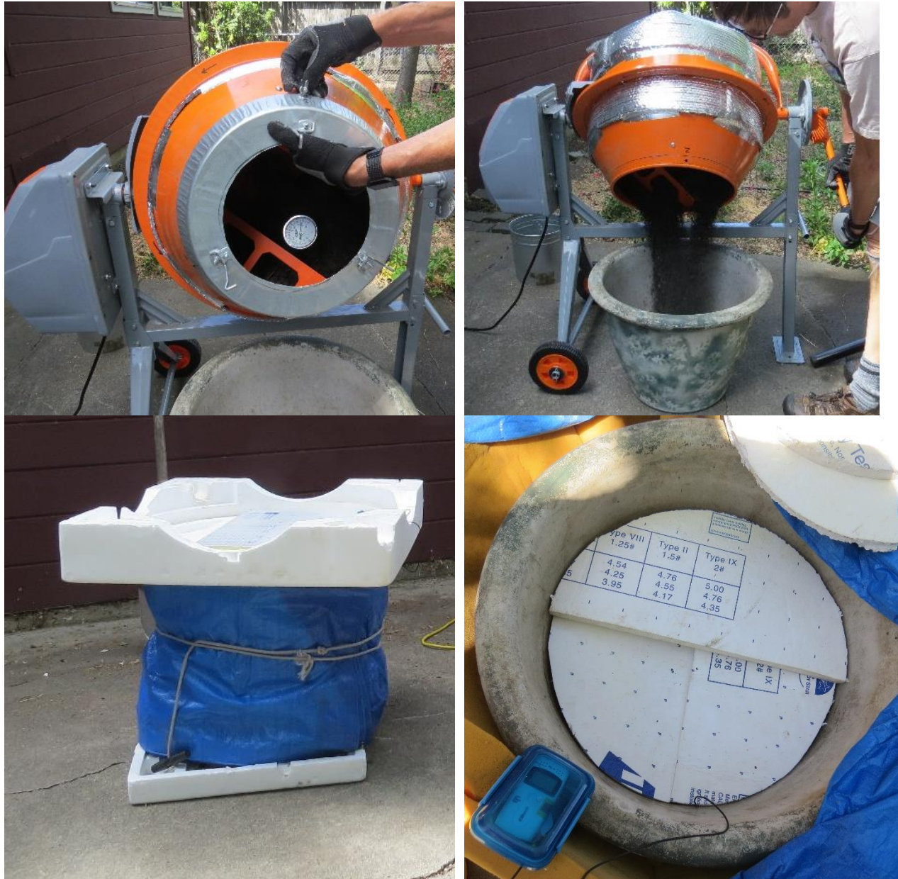
Figure 5. Removing soil from mixer. After the target temperature was reached, the collar on the mixer was removed (top). Both IR and analog thermometers (top) were used to check soil temperature before the soil was transferred. At bottom left, heated soil is transferred into a holding vessel (bottom left). In initial tests (trials 1 - 4), this plastic holding vessel was not insulated and was covered with a piece of polystyrene foam. In later tests (trials 5 - 9), the container was also placed on a polystyrene foam base to insulate it from the underlying concrete. In trials 10 - 20, the sides of the vessel were also insulated with a layer of polyurethane foam wrapped in a polyethylene tarp (lower right). In trials 19 and 20, an additional double layer of foam insulation was placed directly on the soil surface inside of the vessel (bottom right).
