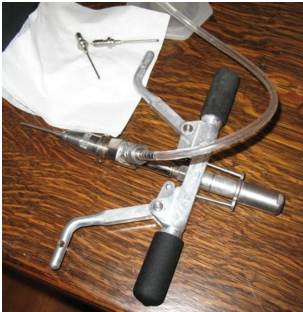
Figure 1. Arborsystems injector and tips.
