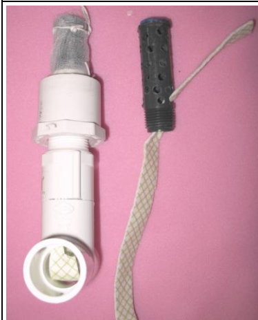
Filter fabric is wrapped around the drain stem and a wick extends from the bottom end of the drain stem to the outside of the column.
