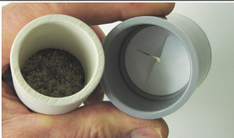
Upper end of filled column showing sand/loam mixture and baffle in intake.
