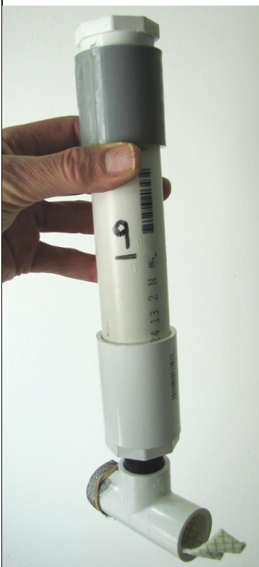
Assembled column with one screen removed and wick pulled out
