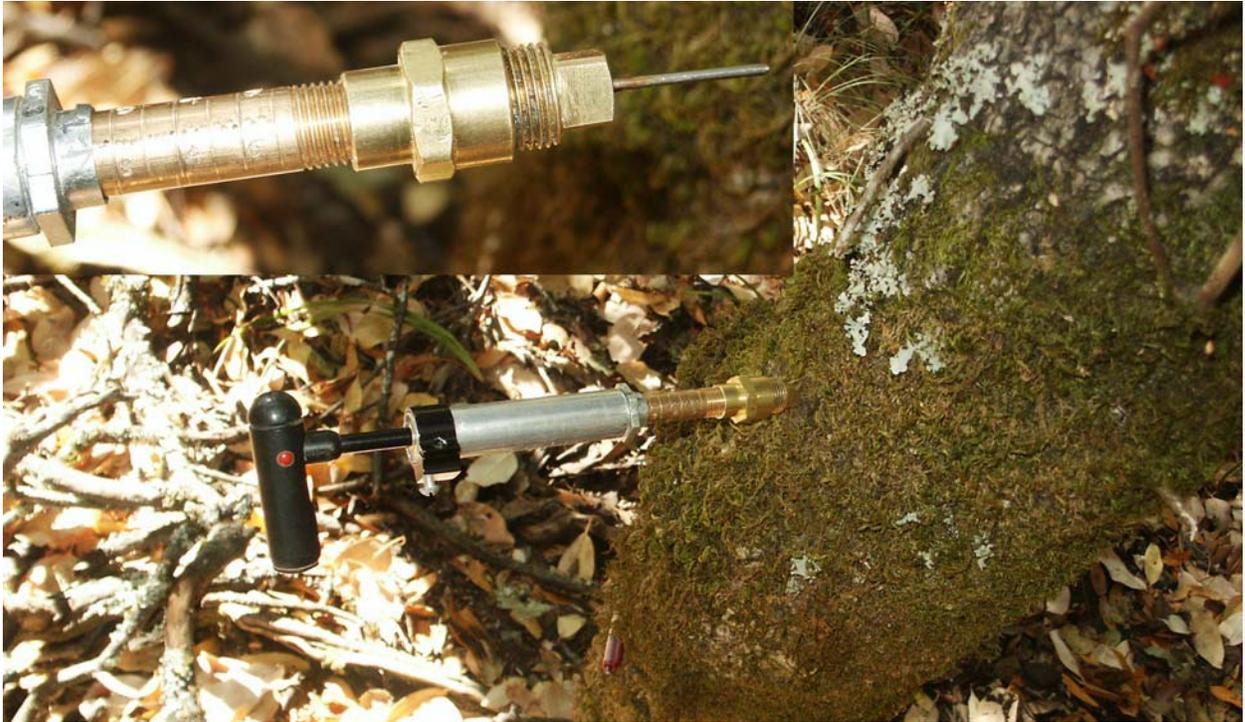
Figure 2. Bark probe used to measure bark thickness, adapted from the design used by Gill and others (1982). The square brass tip of the probe is placed against the surface of the bark and a blunt-tipped 1.9 mm diameter steel probe (constructed from a bicycle tire spoke) is pressed through the bark. The probe tip stops when it reaches the wood and the depth of the probe is read to the nearest mm from gradations engraved in the outer brass barrel of the probe.
